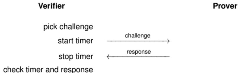
Running at the speed of light:  $10\text{ns} = \text{round-trip of } 2 \times 1.5\text{m} \dots$
